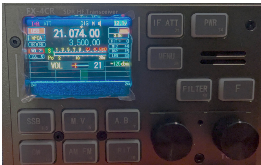
Figure 9: FX-4CR volume knob set between 18–24 maintaining green input levels in WSJT-X.
